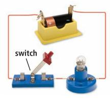
A switch allows you to open and close the circuit without disconnecting any wires.
