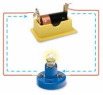
When the parts of the circuit are connected with no gaps, the bulb will light.
