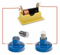
If you remove one part from the circuit, you create a gap. Current no longer moves through any of the parts.
