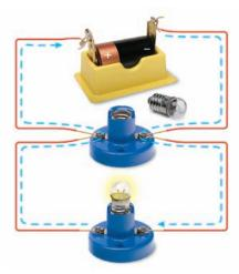
If you remove one part from the circuit, current can still move through the other parts.
